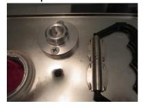
After filling, center the aerosol upside-down on the purge tool and press downward for 3 seconds until only gas escapes, then reinstall put the sprayhead on the aerosol can.
