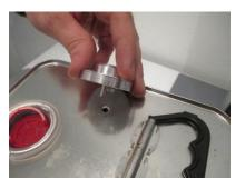
Fix the purging tool in place on the can using the furnished screws.
